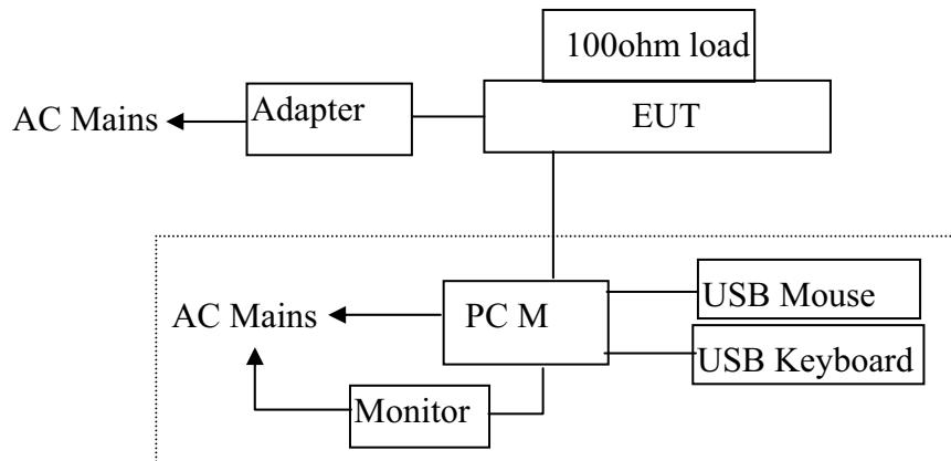
PC M run test software to control EUT work in Tx mode
