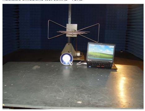
Radiated emissions test > 1GHz
