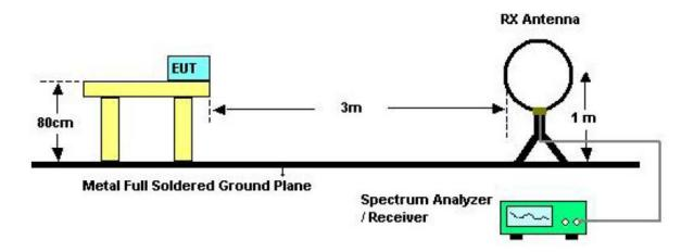
**Below 30MHZ Test setup**
