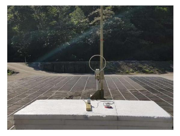
Radiated Measurement Photos (Below 30MHz)
