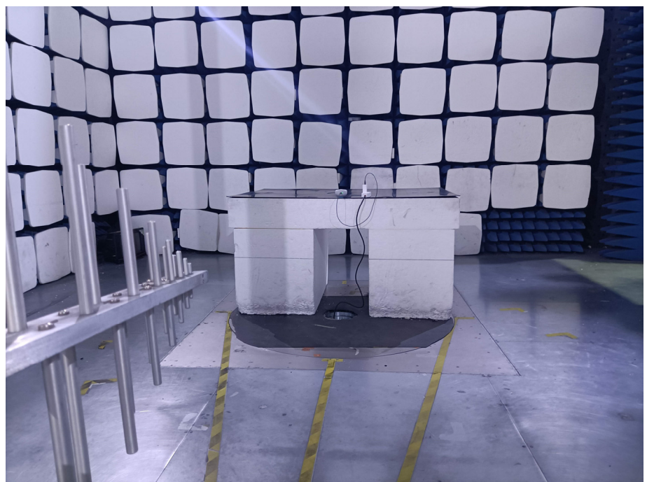
Radiation Emission Test Setup (30MHz to 1GHz)
