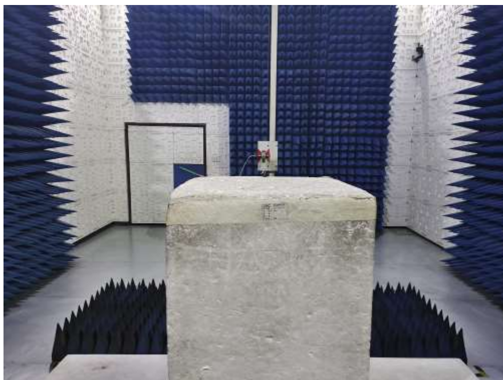
RADIATED EMISSION TEST SETUP ABOVE 1GHz
