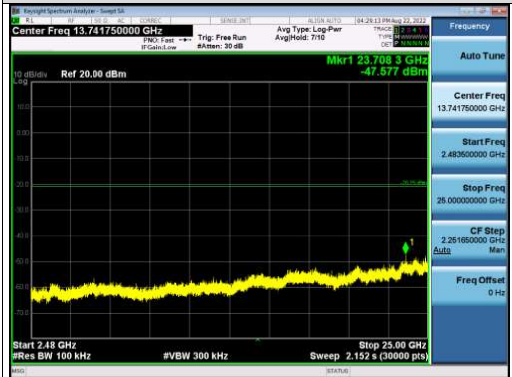
Test_Graph_BR_ANT1_2441_1Mbps_Higher Band Emissions
