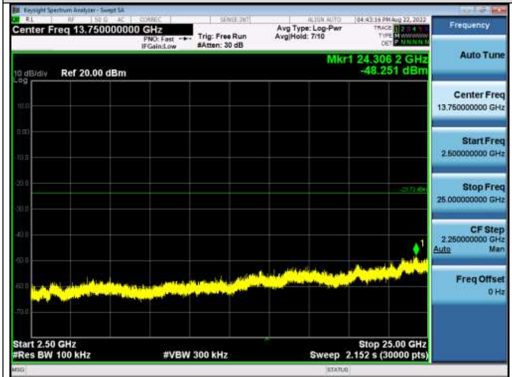
Test_Graph_EDR_ANT1_2480_2Mbps_Higher Band Emissions
