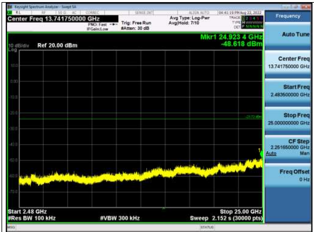
Test_Graph_EDR_ANT1_2441_2Mbps_Higher Band Emissions
