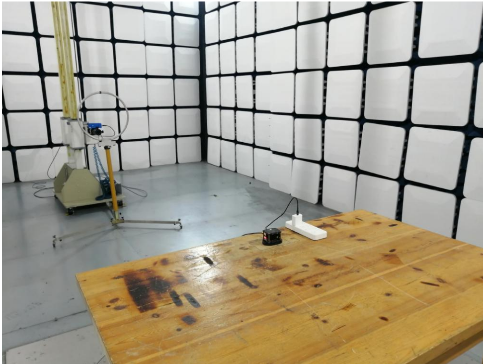
Photo of Radiation Emission Test
