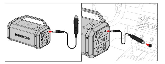
4. The product will start to charge the vehicle battery, it will take about 30 minutes (depends on the vehicle battery size and the power state of the discharged battery) for the vehicle to get enough power to jumpstart.
