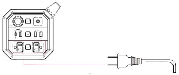
If AC device has short circuit or more power required than the rated output on power station, it will trigger the device to protect itself on short circuit or over load condition.
