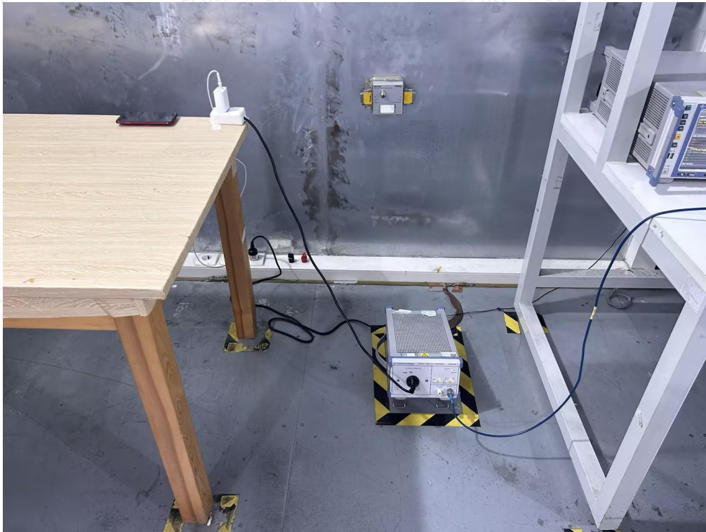
Conducted Emission-AC adapter charge mode
