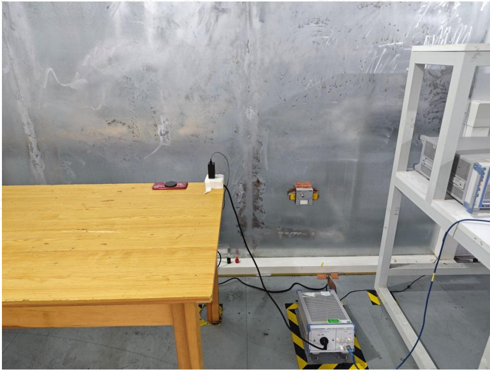
Conducted Emission-AC adapter charge mode
