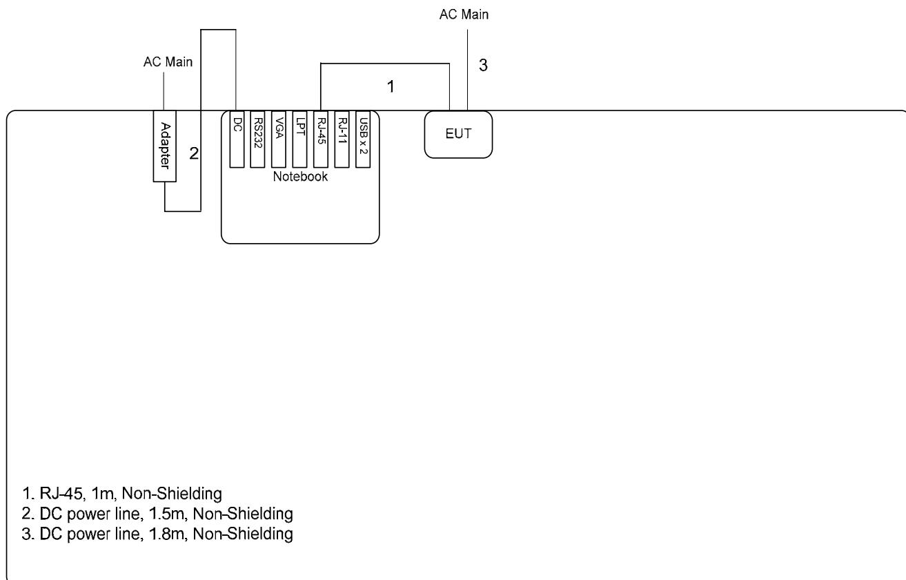
**For radiated emissions above 1GHz**
