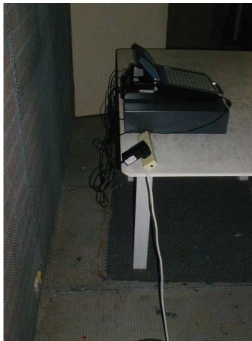
Conducted Disturbance Test Setup (Photo 2)
