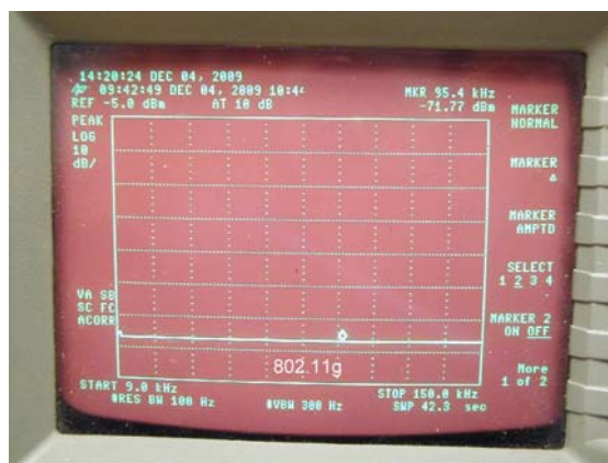
Out-of-Band Emission Plots (802.11g – 9kHz-150kHz)
