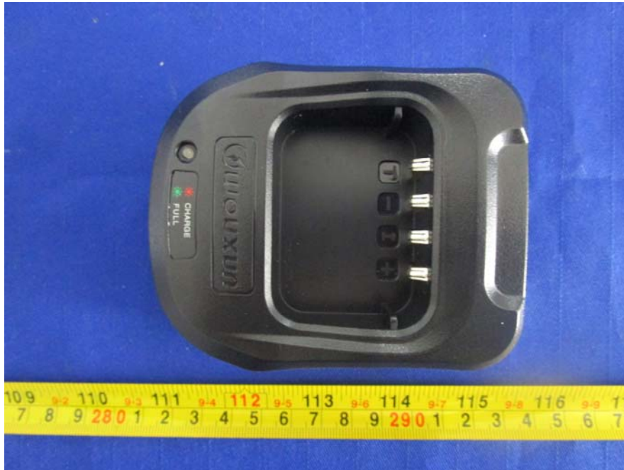
EUT – Charger Top View
