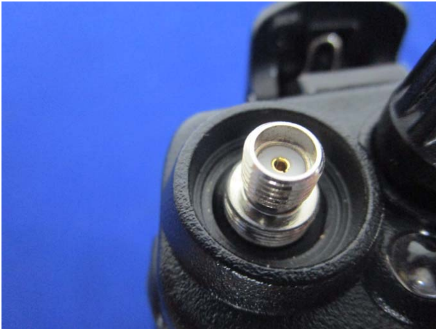
EUT – Antenna Port View
