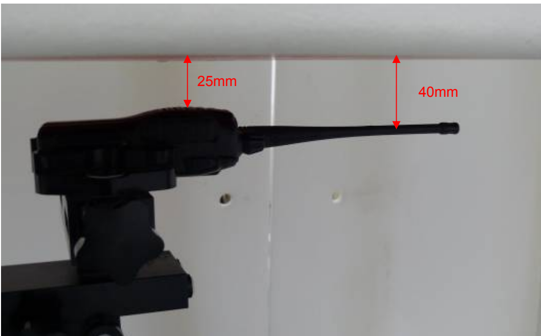
Picture 4: Face-held, The EUT display towards phantom, the distance from EUT Antenna to the bottom of the Phantom is 40mm
