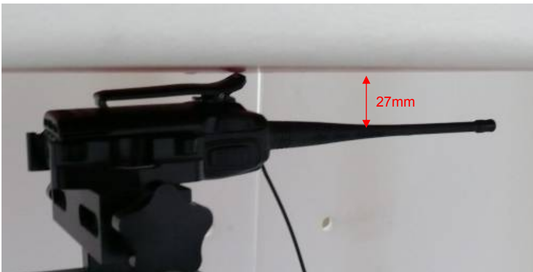
Picture 6: Body-worn with Earphone, The EUT display towards ground, the belt directed tightly to touch the bottom of the flat phantom, the distance from EUT Antenna to the bottom of the Phantom is 27mm
