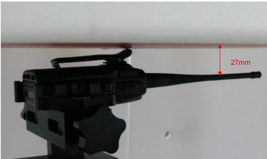
Picture 5: Body-worn, The EUT display towards ground, the belt directed tightly to touch the bottom of the flat phantom, the distance from EUT Antenna to the bottom of the Phantom is 27mm
