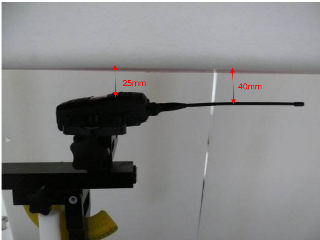
Picture 4: Face-held, the front of the EUT towards phantom, the distance from EUT Antenna to the bottom of the Phantom is 40mm
