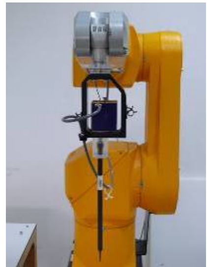
Figure 3. EX3DV4 E-field probe
