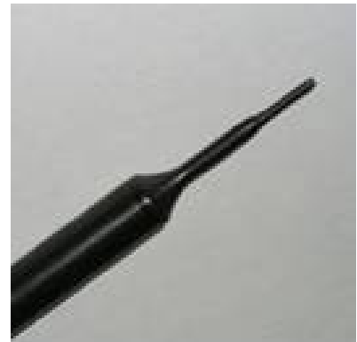
Figure 2. EX3DV4 E-field Probe
