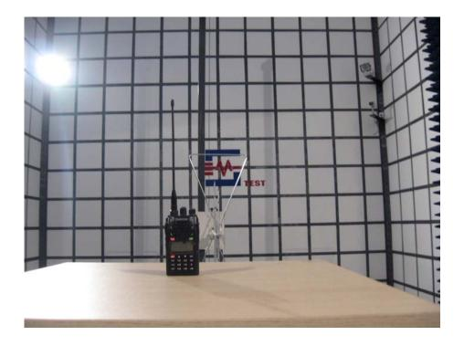
Radiated Spurious Emission Setup 2(Above 1GHz)
