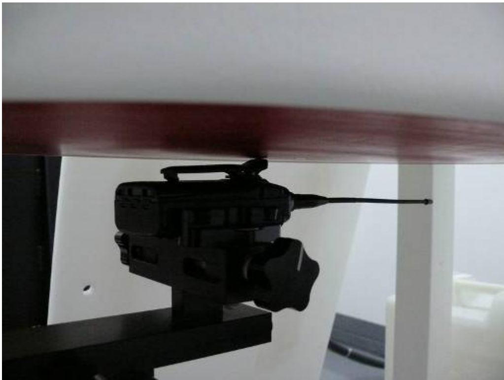
Picture 5: Body-worn, The EUT display towards ground, Belt clip attach the Phantom
