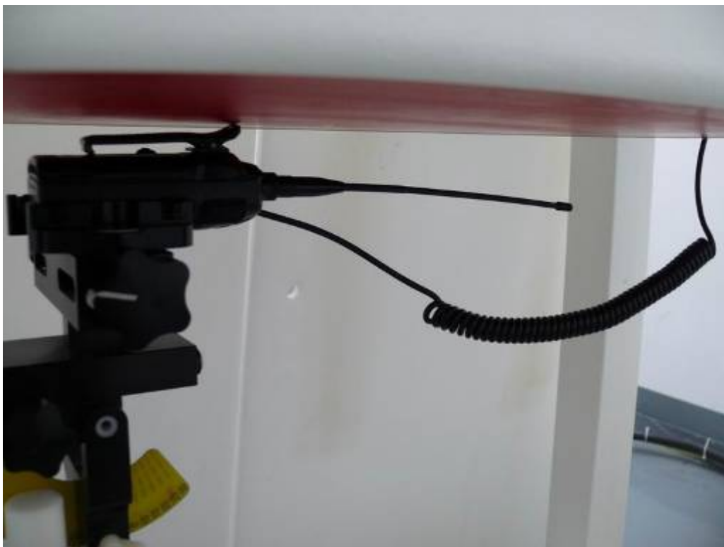
Picture 7: Body-worn with Microphone, The EUT display towards ground, Belt clip attach the Phantom
