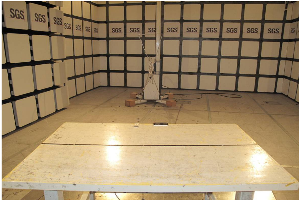
Radiated Emission Test Setup Photo (config 4)
