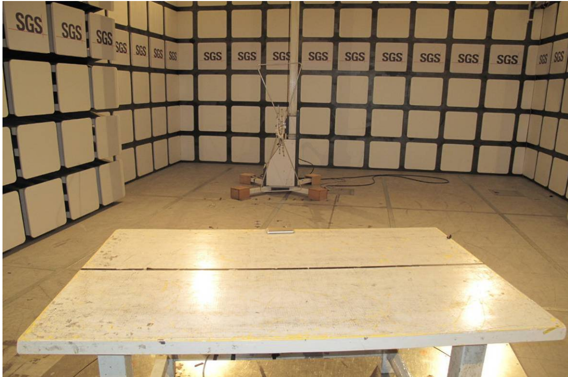
Radiated Emission Test Setup Photo (config 1, 5)
