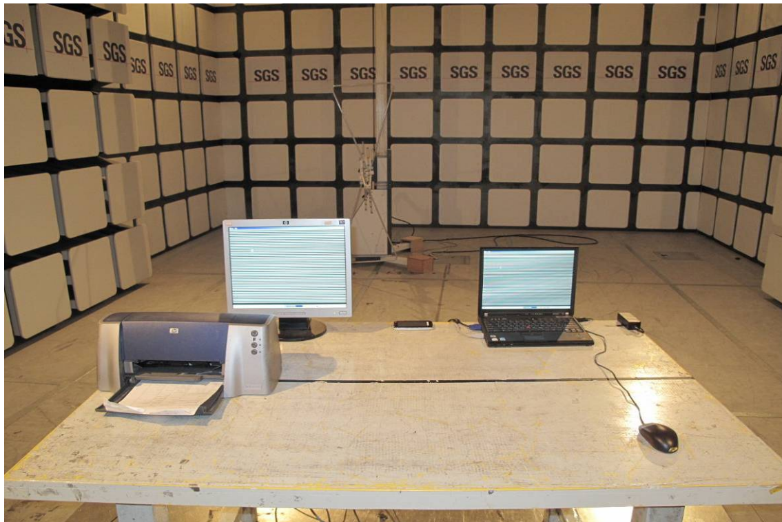
Radiated Emission Test Setup Photo (config 3)
