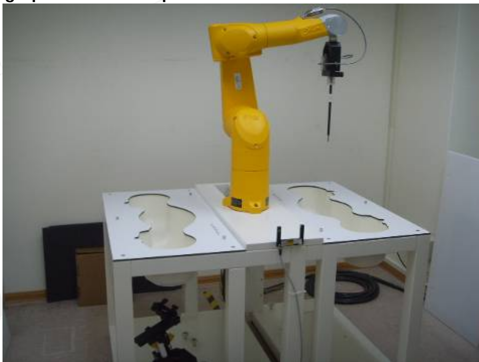
Fig.1 Photograph of the SAR measurement System
