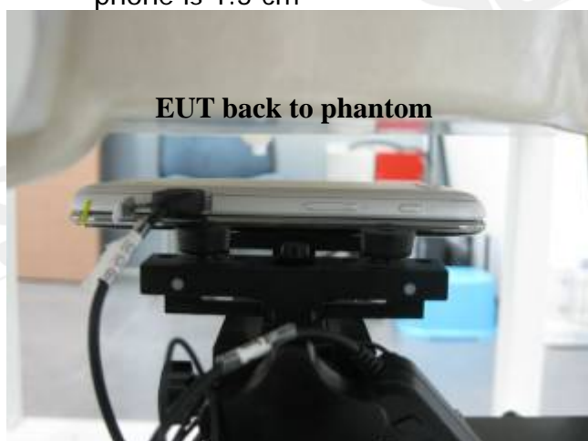
Fig.13 Body worn- EUT back to flat phantom and distance between flat phantom and mobile phone is 1.5 cm with headset.
