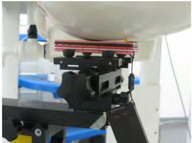
Fig.15 Left Head Section / Cheek-Touch Position_ Slider close repeated with earphone cable case(position 3 & 4)
