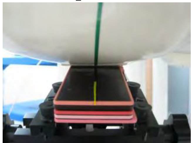
Fig.4 Right Head Section / Ear-Tilt Position(15°)_ Slider close
