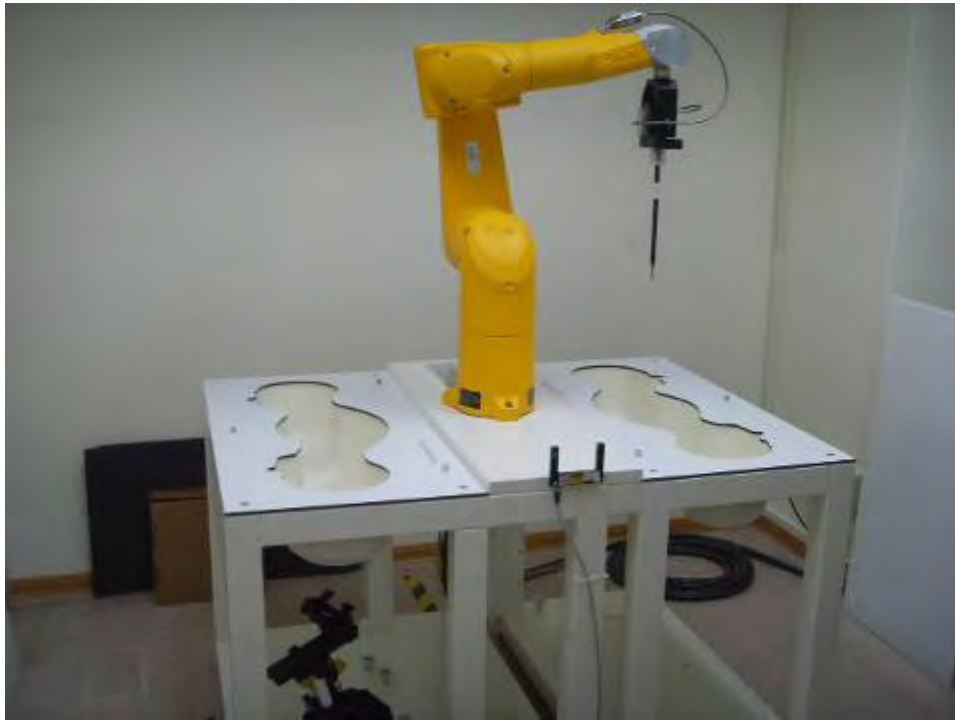
Fig.1 Photograph of the SAR measurement System
