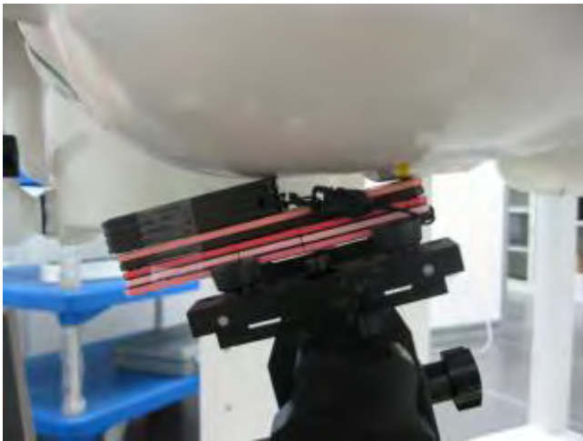
Fig.15 Left Head Section / Cheek-Touch Position_ Slider close repeated with earphone cable case(position 3 & 4)
