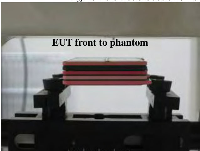
Fig.11 Body worn- EUT front to flat phantom and distance between flat phantom and mobile phone is 1.5 cm
