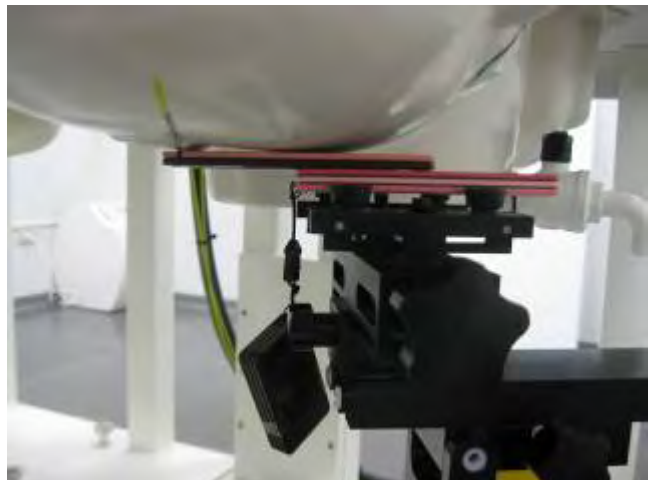
Fig.17 Right Head Section / Cheek-Touch Position_ Slider open repeated with earphone cable case(position 3 & 4)
