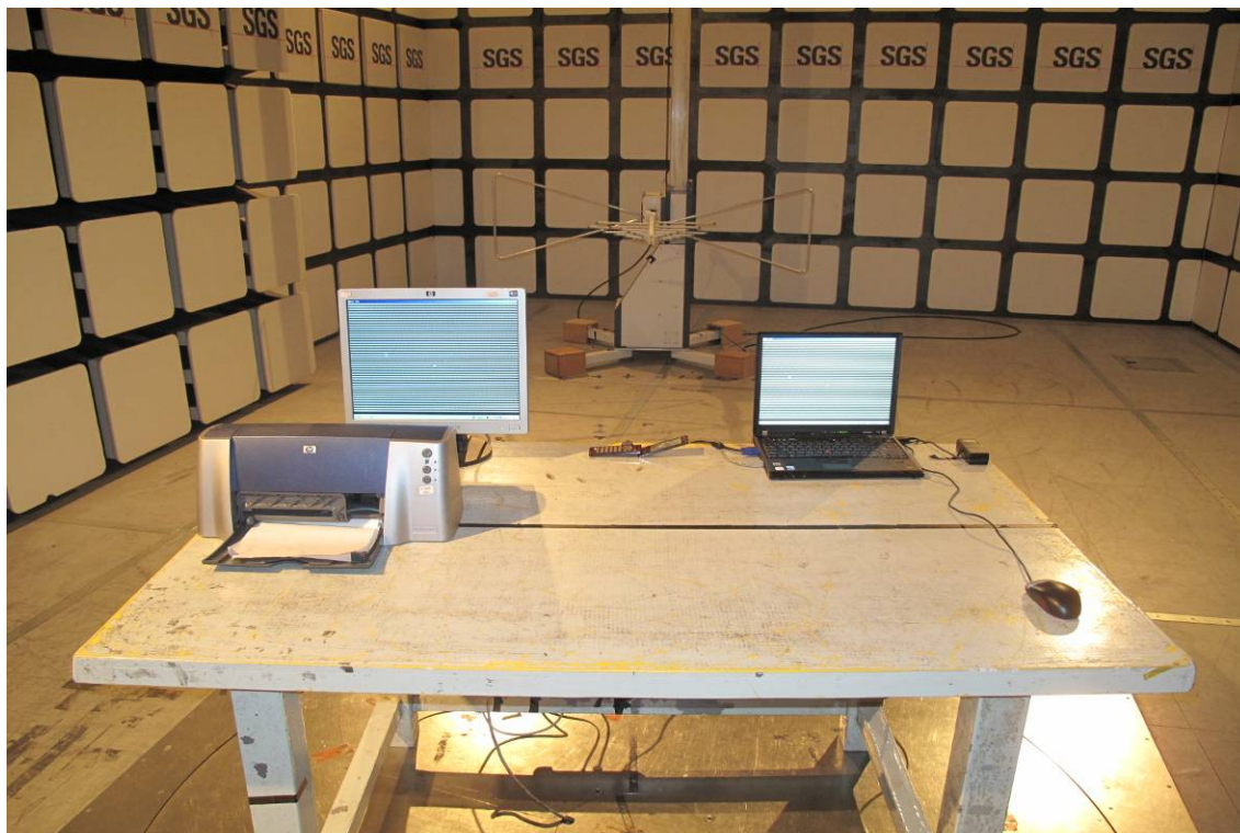
Radiated Emission Test Setup Photo (config 5)
