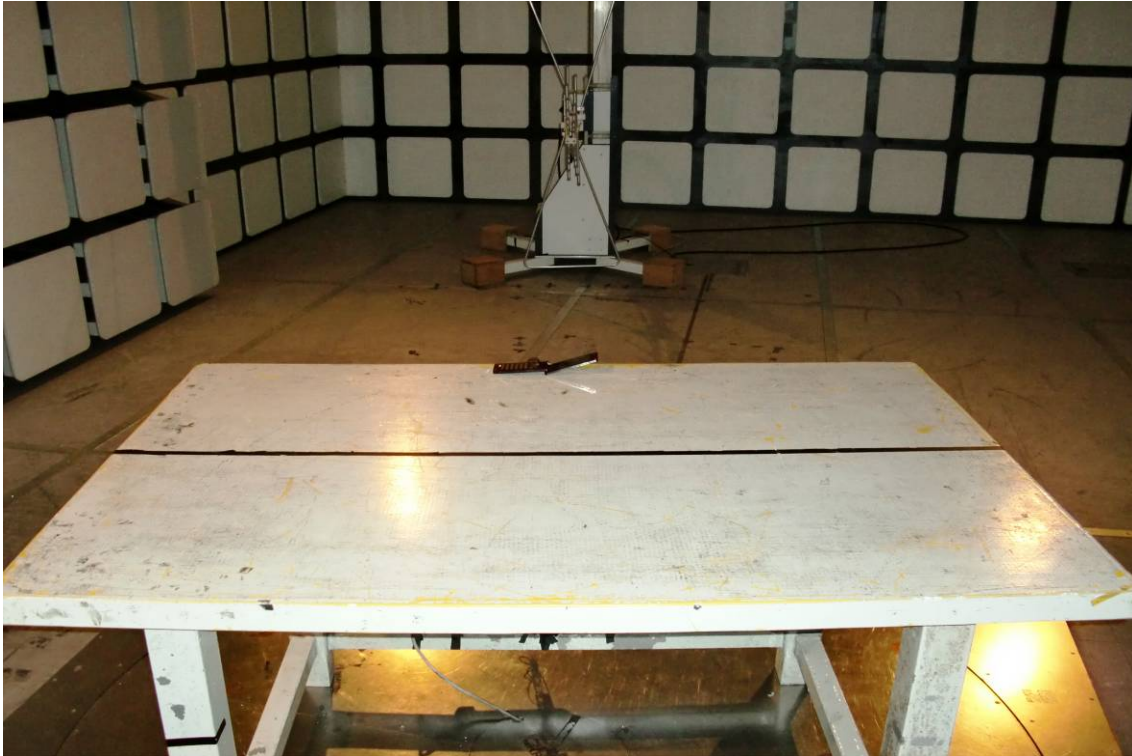
Radiated Emission Test Setup Photo (config 1, 3)
