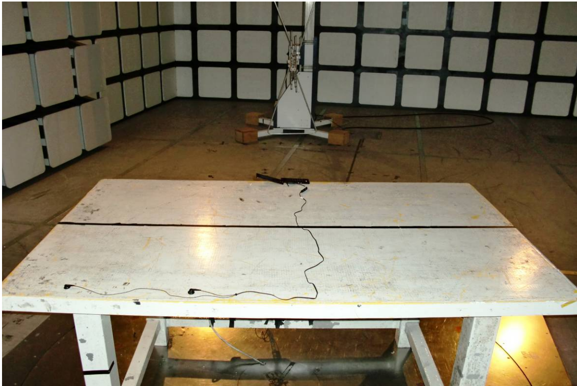
Radiated Emission Test Setup Photo (config 2, 4)
