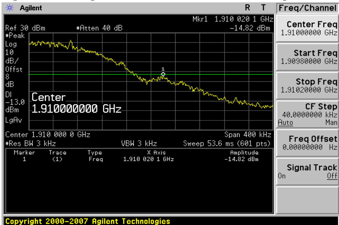
Figure 8-10: Band edge emission at antenna terminals –PCS 1900 Highest Channel
