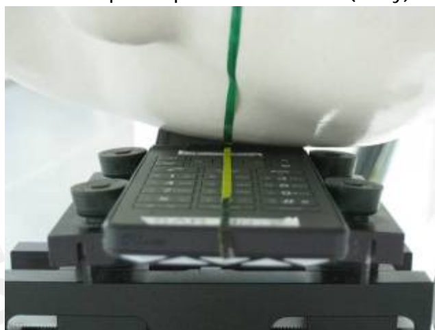
Fig.3 Right Head Section / Cheek-Touch Position
