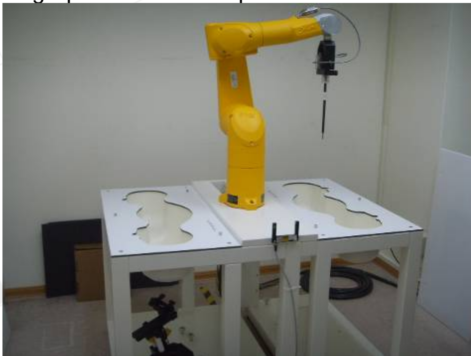
Fig.1 Photograph of the SAR measurement System
