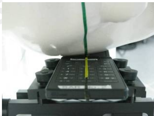
Fig.5 Left Head Section / Cheek-Touch Position
