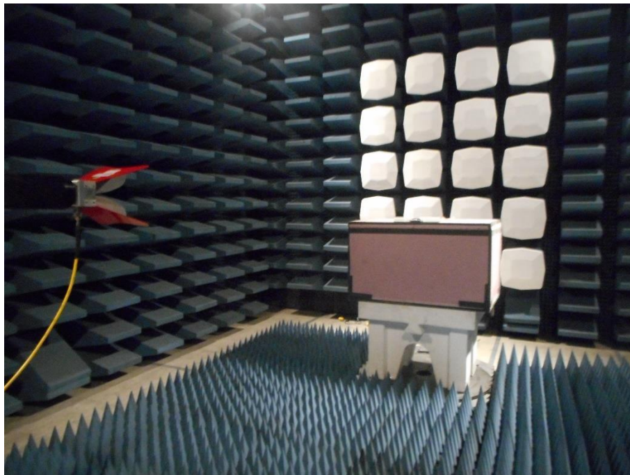
Radiated Emission test setup in Semi Anechoic Chamber (above 1GHz)
