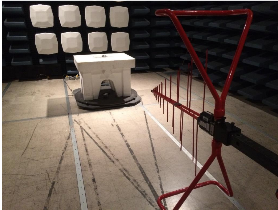
Figure 1: Radiated Spurious Emissions performed at the SAC Test Setup
