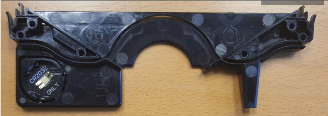
Verilock RbA CSMT PCB in Carrier – FRONT (with cover)
