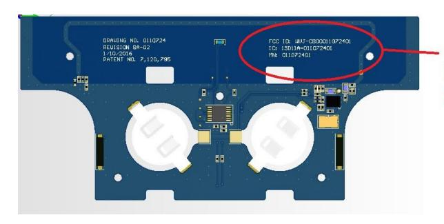
FCC and IC Identifications are printed directly onto the PCB, and is in plain view for the user when installing batteries.
