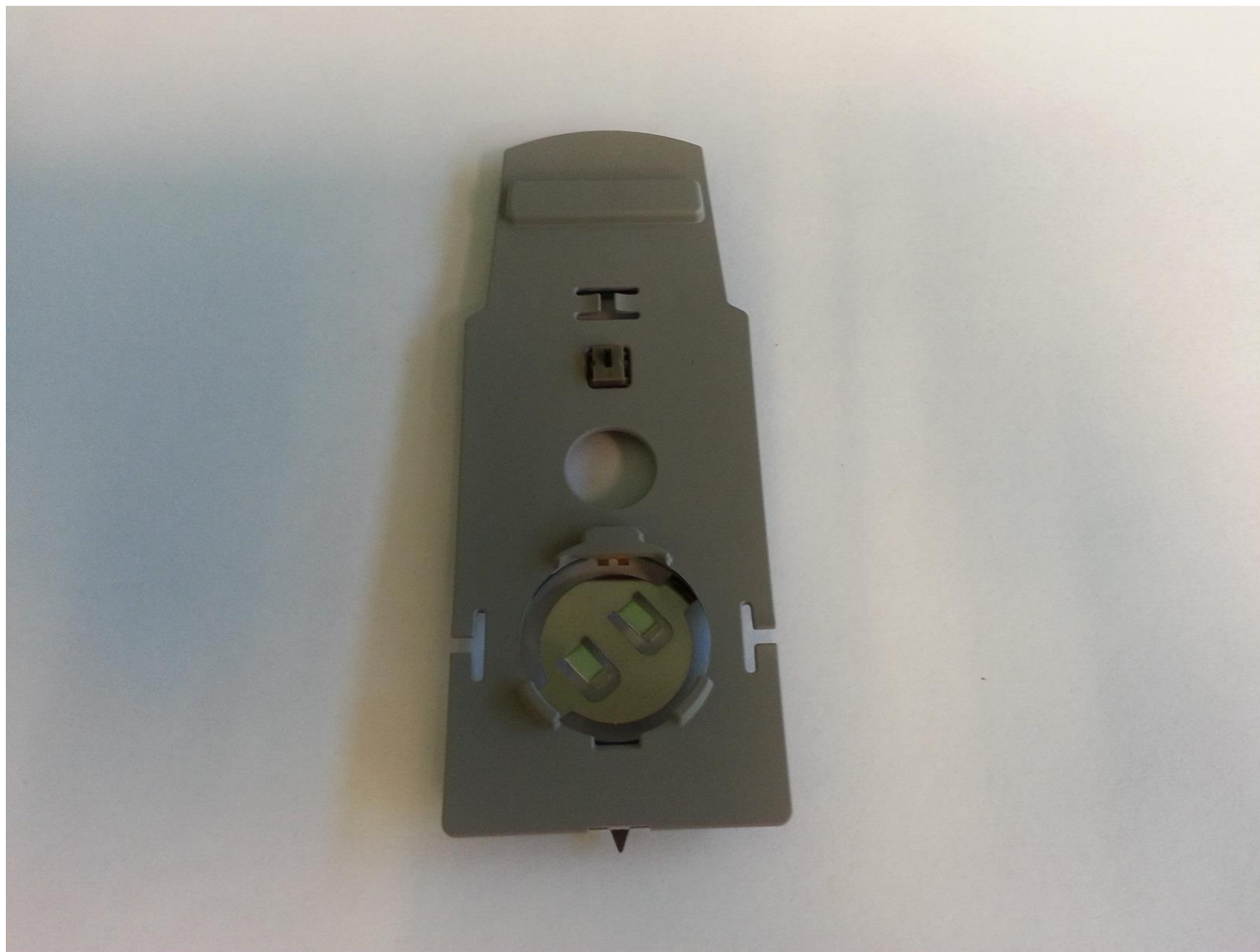
Gliding Door – PCB Assembly in Plastic Carrier – BACK
