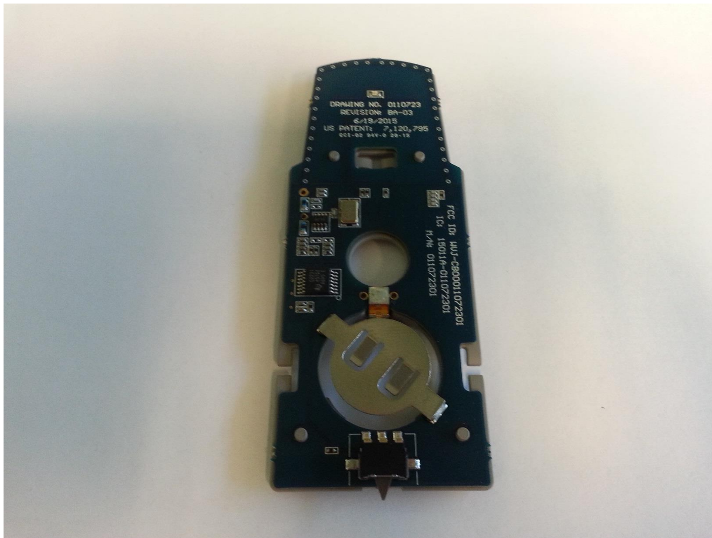
Gliding Door – PCB Assembly in Plastic Carrier - FRONT
