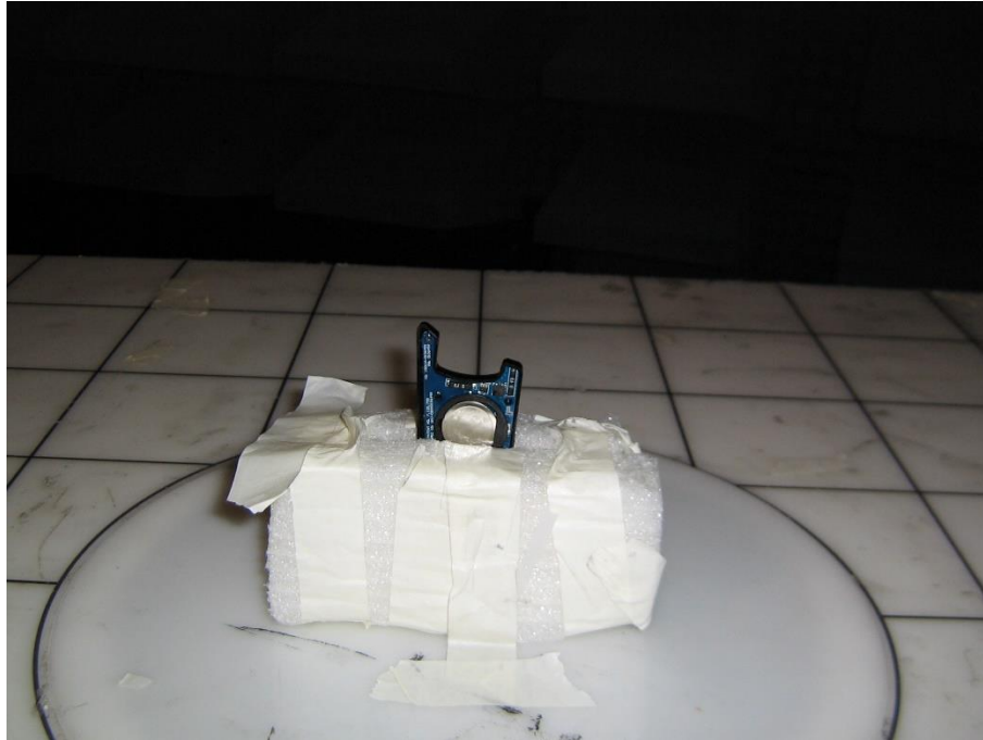
Radiated Emission test setup in Semi Anechoic Chamber
