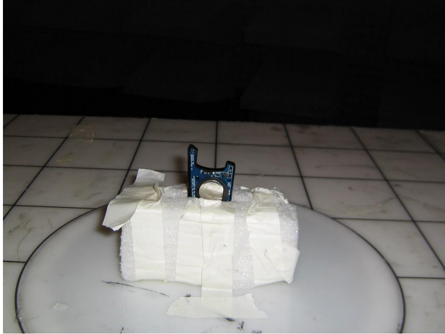
Radiated Emission test setup
