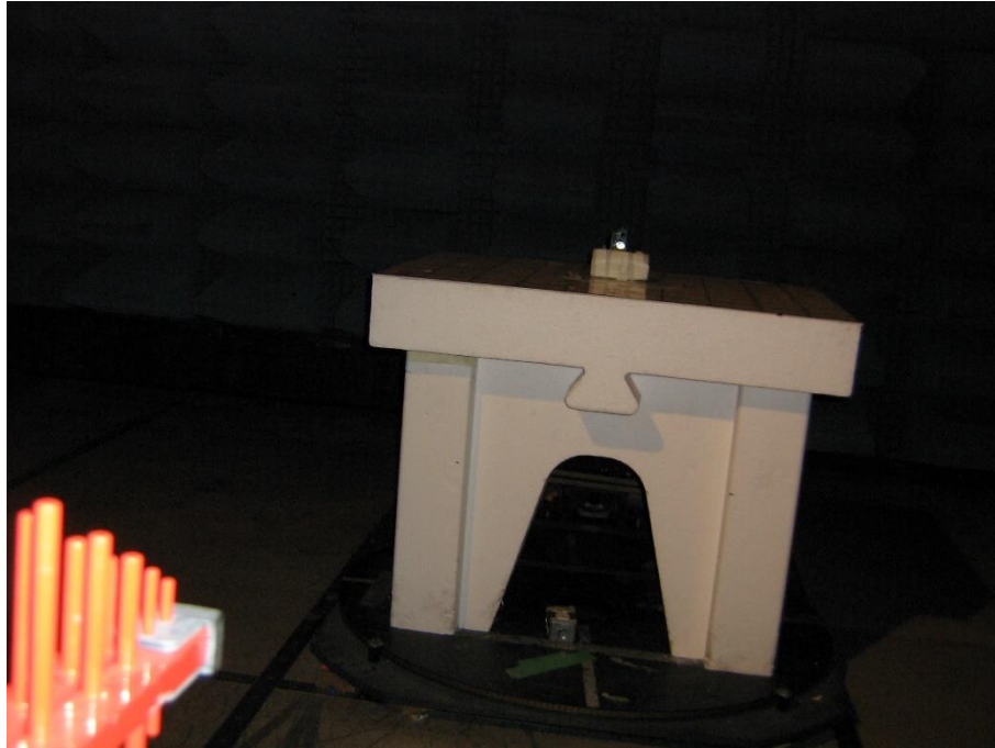
Radiated Emission test setup in Semi Anechoic Chamber – 30MHz - 1GHz
