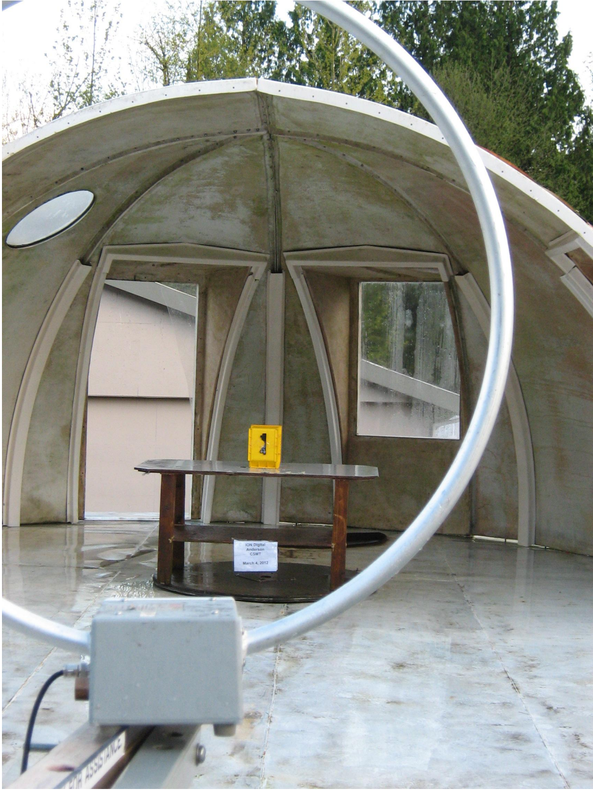
Test Setup for Spurious Radiated Emissions Frequencies below 30 MHz
