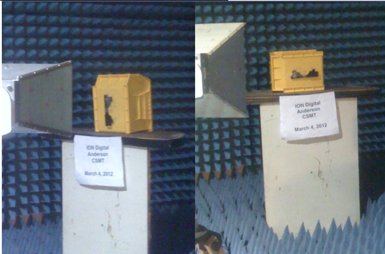
Test Setup for Spurious Radiated Frequencies 1 to 18 GHz.
