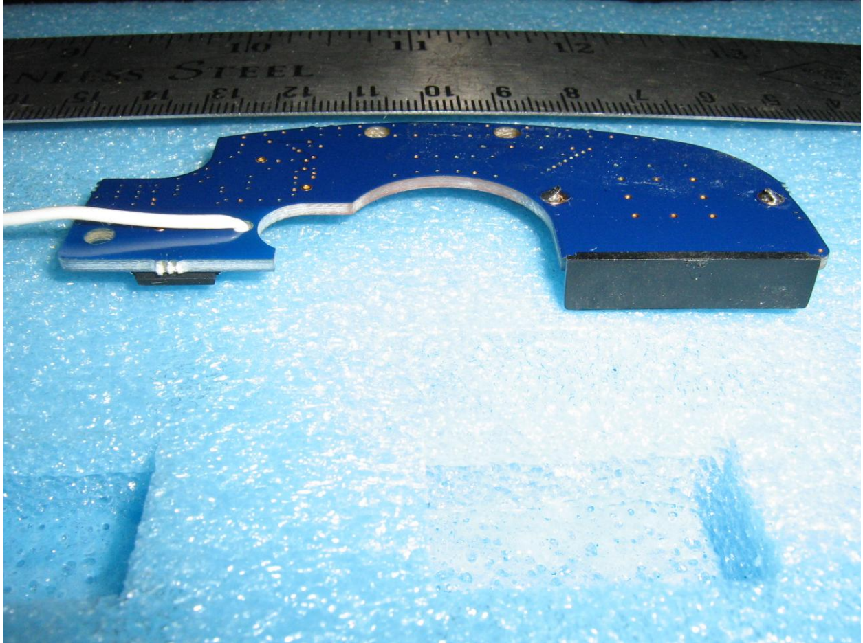
Figure 3 DH rev BB external battery down pcb with battery housing
