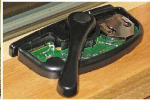
Double-hung lock showing VeriLock™ integrated security sensor
