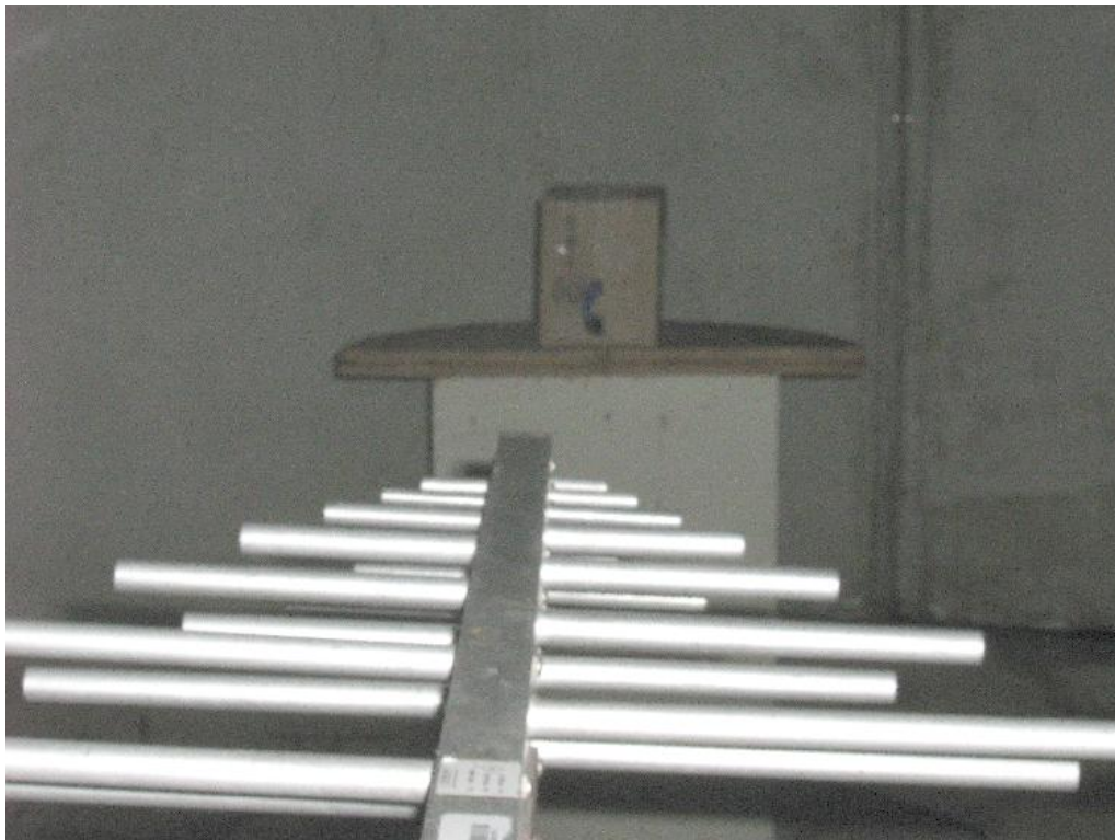
Test Setup for Spurious Radiated Frequencies above 30MHz
