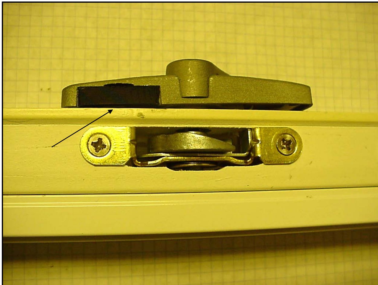
Photograph 4: PCB Inside Locking Mechanism
