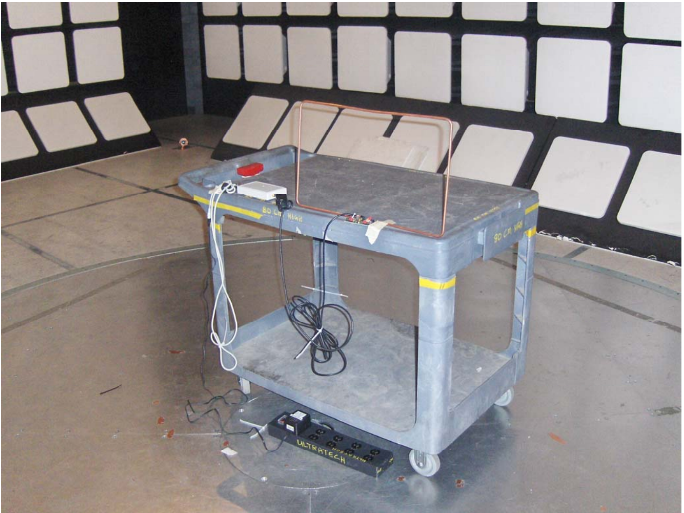
Radiated Emission at 10 m Distance Test Configuration 2: EUT with RML-HFANT500/300-B Inductive Loop Antenna
