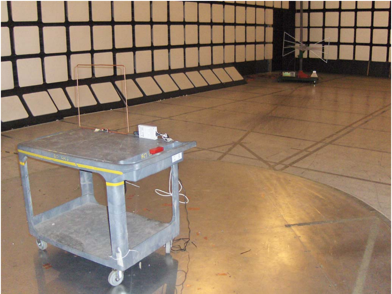
Radiated Emission at 10 m Distance (30 – 1000 MHz) Test Configuration 1: EUT with RML-HFANT500/500-B Inductive Loop Antenna
