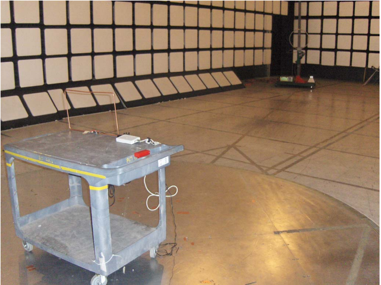
Radiated Emission at 10 m Distance (Below 30 MHz) Test Configuration 2: EUT with RML-HFANT500/300-B Inductive Loop Antenna
