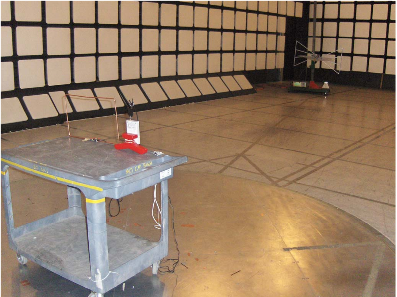
Radiated Emission at 10 m Distance (30 – 1000 MHz) Test Configuration 2: EUT with RML-HFANT500/300-B Inductive Loop Antenna
