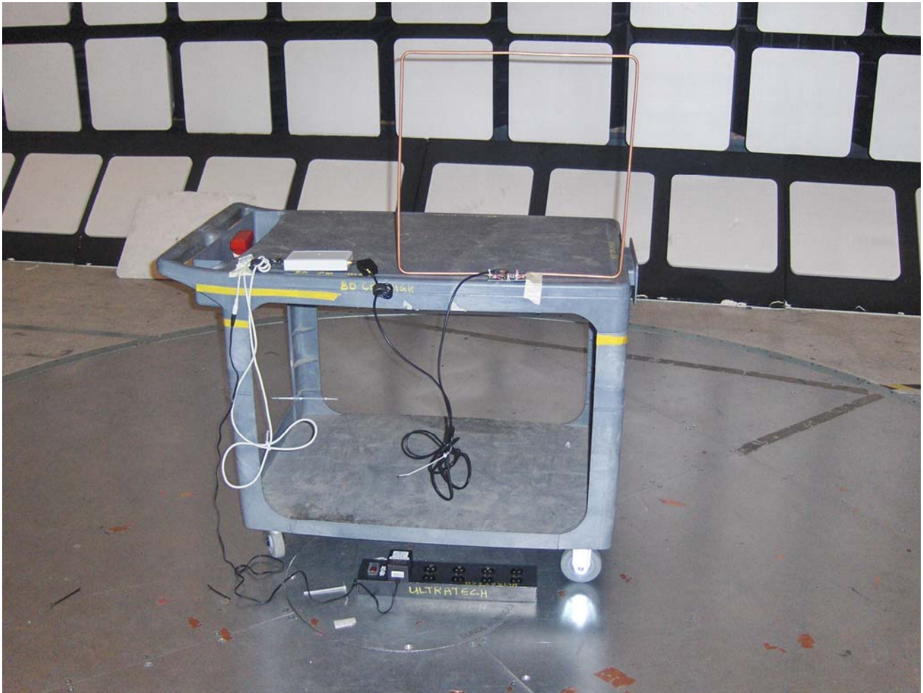
Radiated Emission at 10 m Distance Test Configuration 1: EUT with RML-HFANT500/500-B Inductive Loop Antenna
