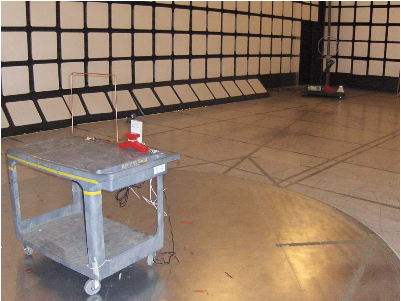
Radiated Emission at 10 m Distance (Below 30 MHz) Test Configuration 1: EUT with RML-HFANT500/500-B Inductive Loop Antenna
