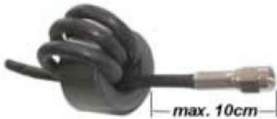
Fig 4: Toroid integration to the coax cable
