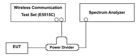
(Configuration of conducted Emission measurement) Test Procedure
