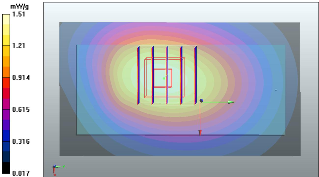
**#12 GSM850\_GPRS10\_Bottom\_1.5cm\_Ch189\_2D****DUT: 140601**
