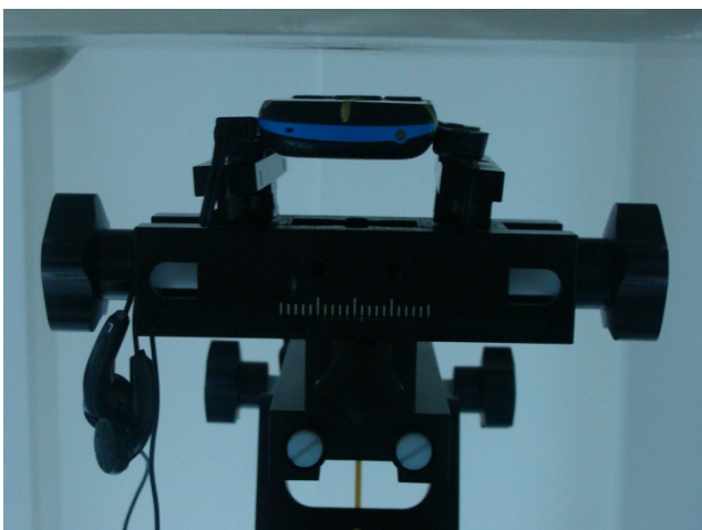
Front of the DUT with Phantom 1.5 cm Gap (with Headset)
