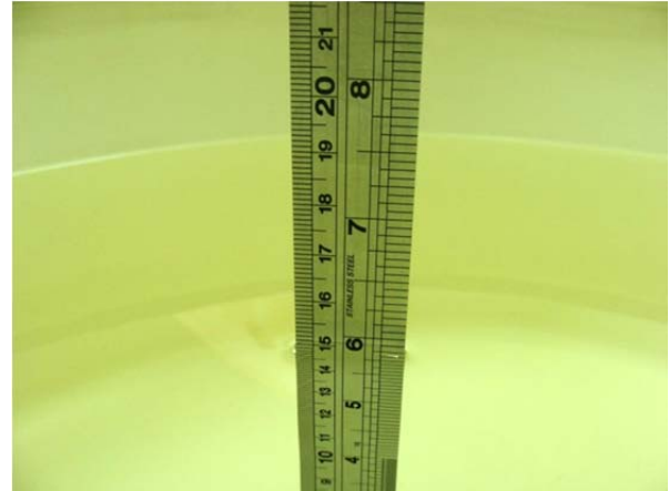
Fig 6.2 Photo of Liquid Height for Body SAR
