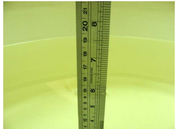
Fig 6.2 Photo of Liquid Height for Body SAR
