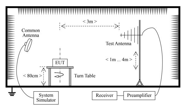
The test is performed in a 3m Semi-Anechoic Chamber; the antenna factor, cable loss and so on of the site (factors) is calculated to correct the reading. The EUT is placed on a 0.8m high insulating Turn Table, and keeps 3m away from the Test Antenna, which is mounted on a variable-height antenna master tower. The Common Antenna is used for the call between the EUT and the System Simulator (SS).
