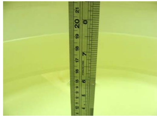
Fig 6.2 Photo of Liquid Height for Body SAR
