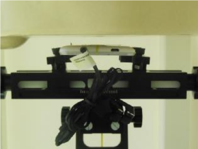
Back with Headset , Test Separation 10 mm
