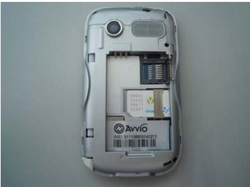
To install the T-Flash card, open its latch.
