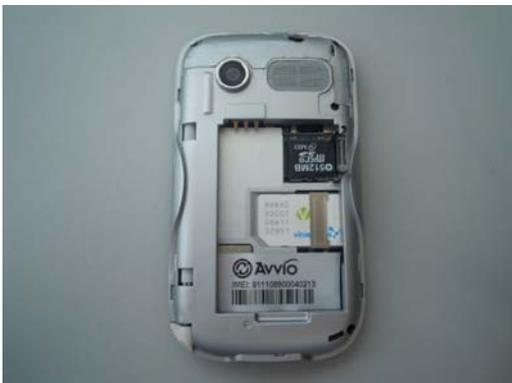
Place its indented side downward, insert the card into the card slot.
