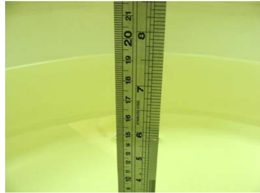
Fig 6.2 Photo of Liquid Height for Body SAR
