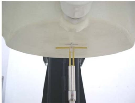
Fig 7.2 Photo of Dipole Setup
