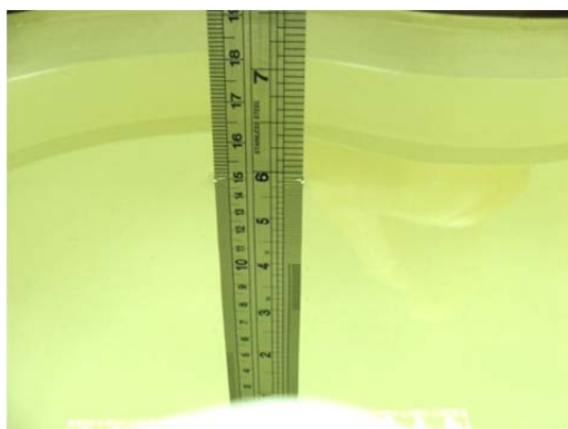
Fig 6.1 Photo of Liquid Height for Head SAR
