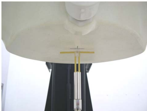
Fig 7.2 Photo of Dipole Setup
