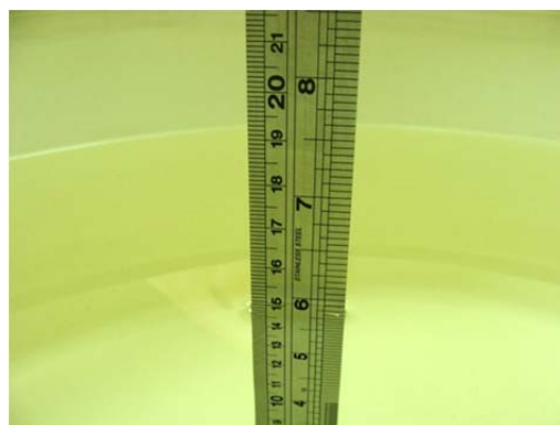
Fig 6.2 Photo of Liquid Height for Body SAR
